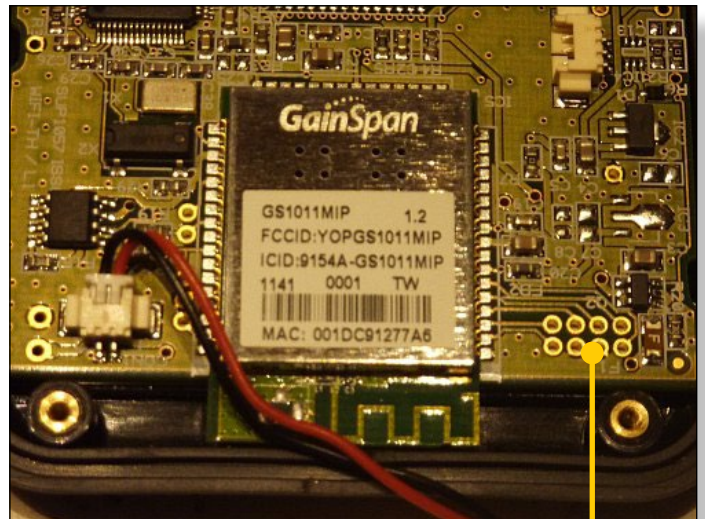
Figure 5 The Wifi adapter module mounts to the logger's main board.
