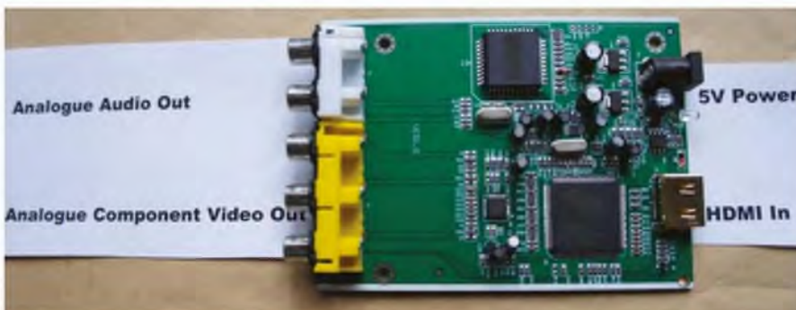
A cheap and easy-to-use HDCP copy-protection-stripping board, easily available from Amazon
