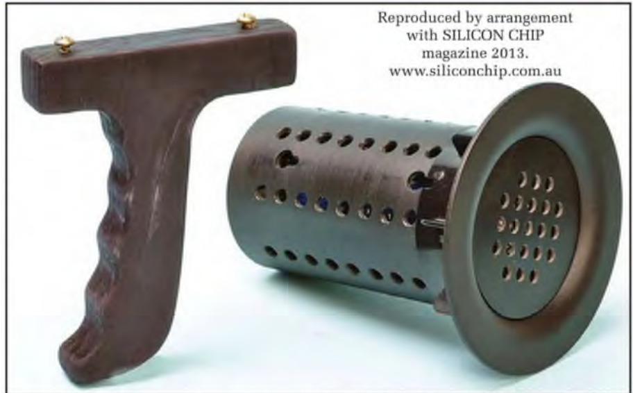
Here's the handle we made – it mates with the two 'keyholes' in the Interplanetary Voice case. Note also the drilling required in the case
