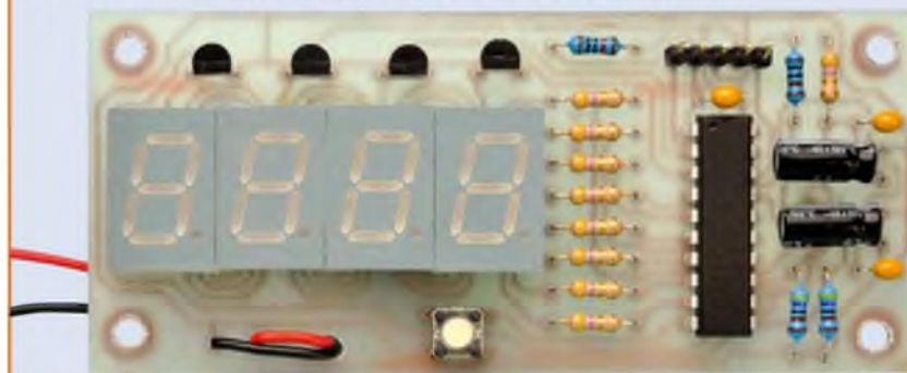
This prototype differs slightly from the final version shown in Fig.3 (eg, Q1 is oriented differently and the hole for the battery leads has been moved)
