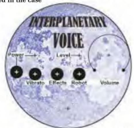
Fig.5: here's the 'front panel' label which also serves as a drilling template. This can be downloaded from the EPE website
