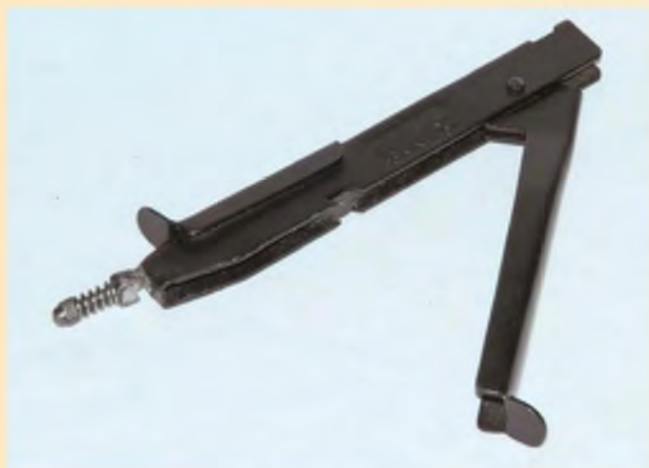
Fig.3. A hand nibbler can quickly cut through most thin sheet materials. A tool of this type can be used to produce large cut-outs very quickly, but it cannot be used to make curved cuts
