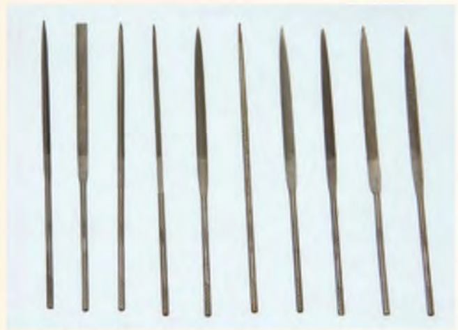
Fig.2. 'Needle' files are often sold in sets containing a variety of shapes. A round type is all that is needed for making cut-outs, but other types are useful for tidying cut-outs
