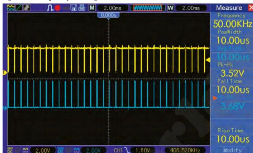
Fig.5: this third capture of USB signal waveforms is at a much slower rate again, and shows the way the D+/D- data packets are sent at intervals of 1ms. Again, the frequency reading is not relevant.
