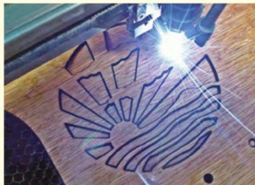
Fig.17. Laser cutting the retro-design radio enclosure
