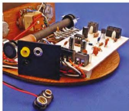
Fig.15. Rear bracket with antenna, ground and headphone connectors
