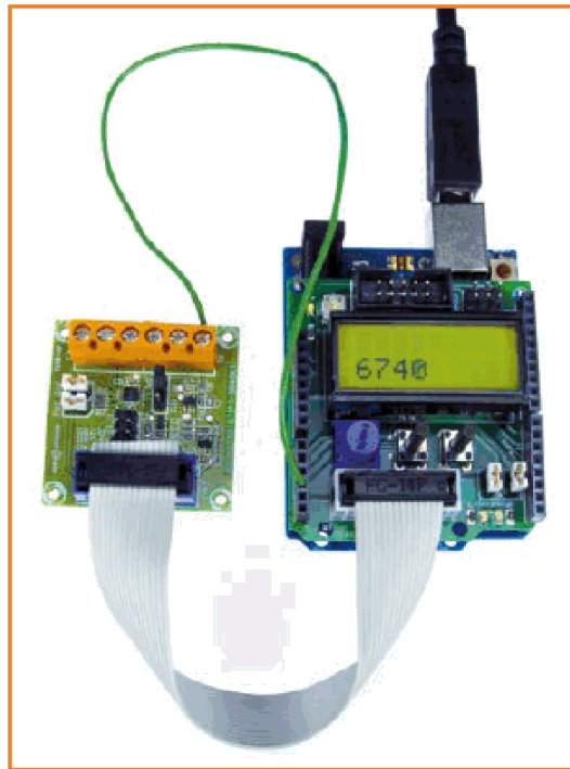
Figure 4. To test the ADC module and the Data logger application connect a wire from the Arduino pin A3 to the ADC input at AINO.
