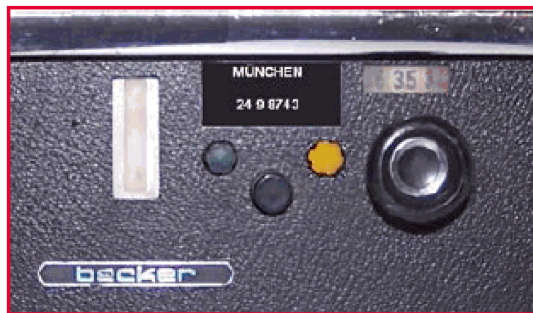
Figure 8. The standard AT400-series "Becker" control box type for dashboard mounting. Still a bit unpolished! (courtesy and copyright oebl.de)
