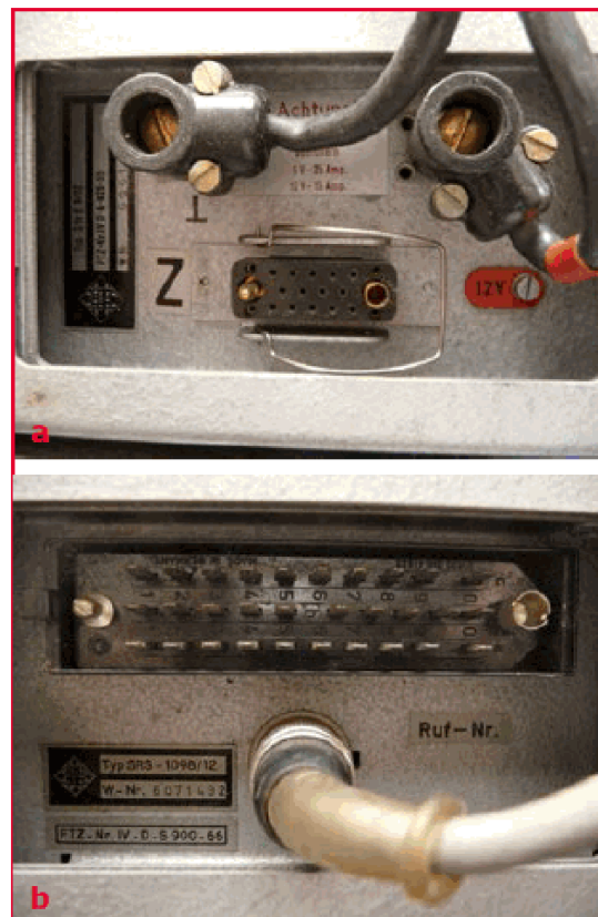
Figure 4. Views of the connector area on the power supply unit STV E 6/12 (4a) and the selcall unit SRS-1098/12 (4b). Ruf-Nr = selcall ident.
