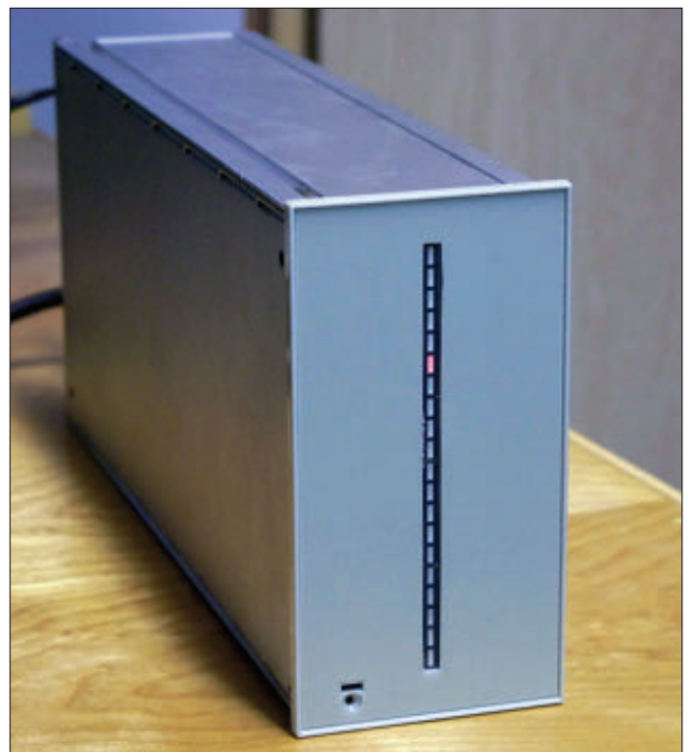
■ FIGURE 11. The controller — which has an LED bar graph display — was built into the box of a surplus oscilloscope plug-in module.
