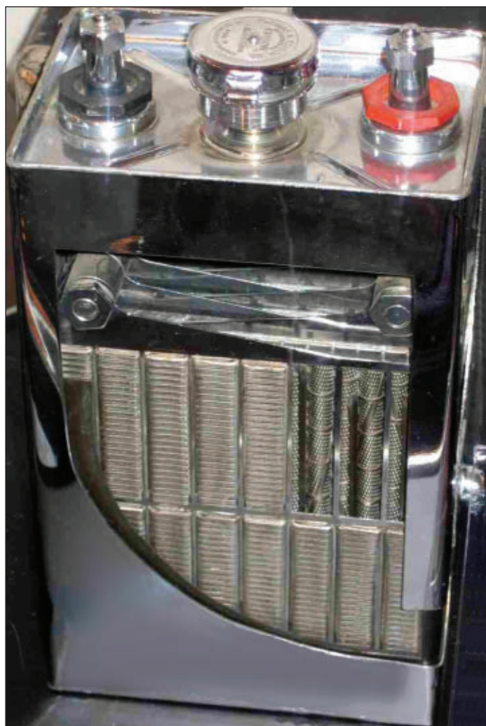
FIGURE 1. Edison cell cut-away. (Photo courtesy of John DeArmond.)
