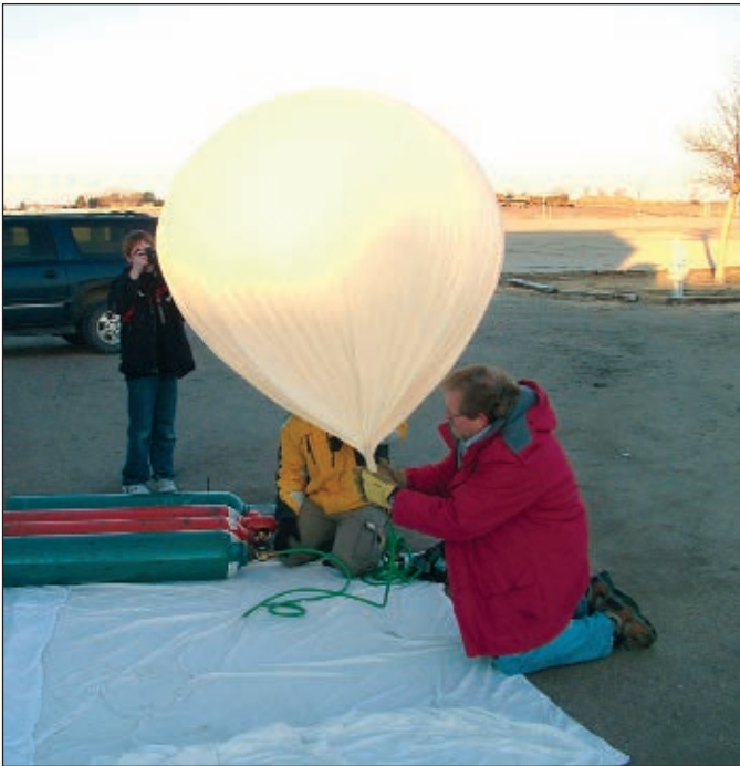
■ FIGURE 2. Dr. Adams is filling the Fort Hays weather balloon with helium. The bed sheet below him protects the balloon from debris on the ground. The filler he is using is a green oxygen hose attached to the least expensive regulator I could find at a welding supply store. The valve on the helium tank (and not the regulator) is controlling the flow of helium into the balloon.
