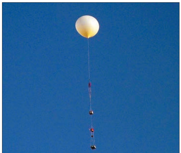
■ FIGURE 4. What a pretty sight! The balloon, recovery parachute, and four payload modules are visible in this image. The cord between the balloon and parachute is the load line and is around 15 feet long. That way, what's left of the balloon falls over the parachute rather than on top of it.
