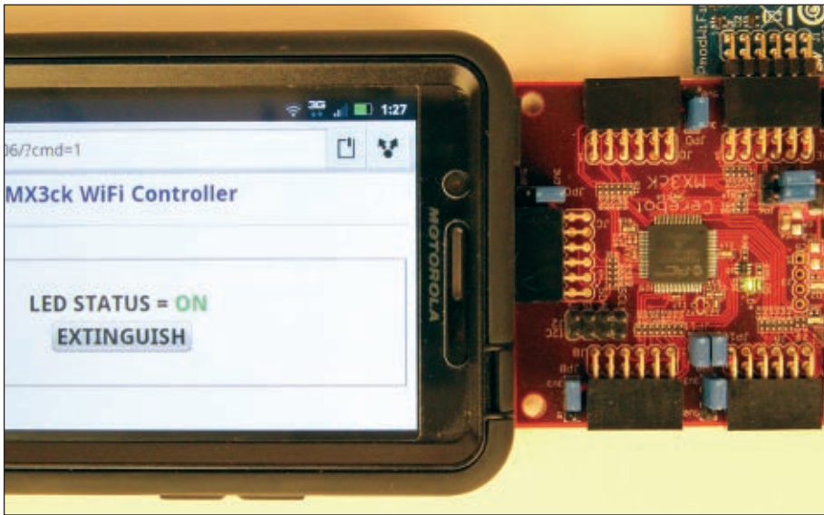
■ PHOTO 3. It's ON! Note the LED is illuminated just to the right of the PIC.
