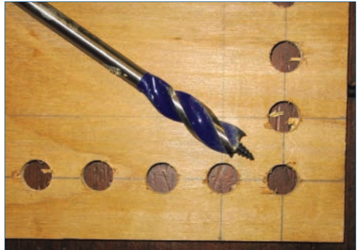
■ FIGURE 9. LED holes drilled in plywood.
