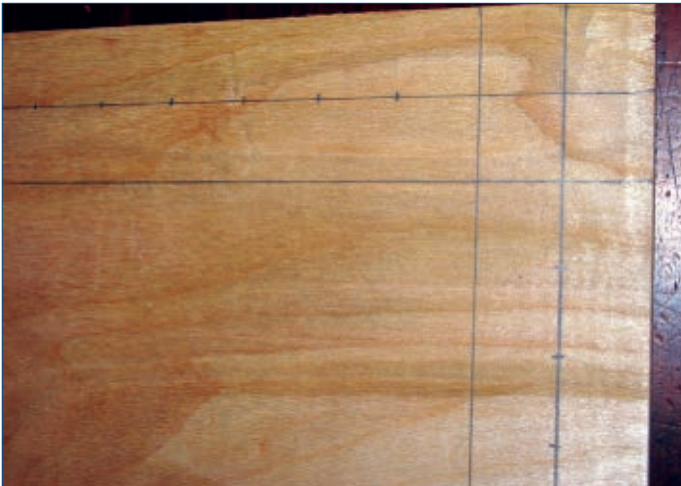
■ FIGURE 8. Frame dimensions transferred to plywood.
