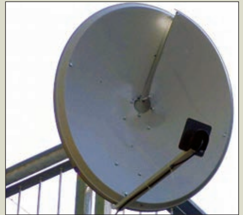
■ Helicoidal parabolic antenna used for the twisted radio waves.
