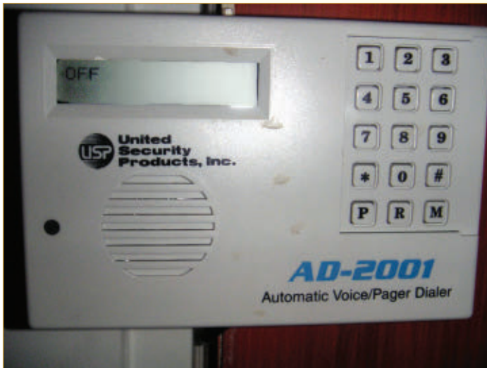
FIGURE 5. COMMERCIAL PHONE DIALERS SUCH AS THIS ONE MAKE IT EASY FOR YOUR HOME TO CALL YOU AND YOUR NEIGHBORS WHEN AN INTRUDER HAS BEEN DETECTED.
