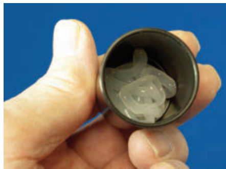
■ FIGURES 10, 11, and 12. Use clear silicone caulk to anchor the PCB in the film can, then apply a moisture seal around the Sonalert unit.
