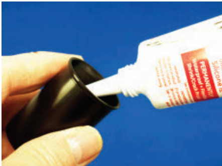
■ FIGURES 10, 11, and 12. Use clear silicone caulk to anchor the PCB in the film can, then apply a moisture seal around the Sonalert unit.
