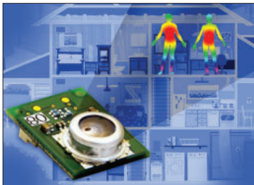
■ Omron's D6T senses human presence without the need for movement.
