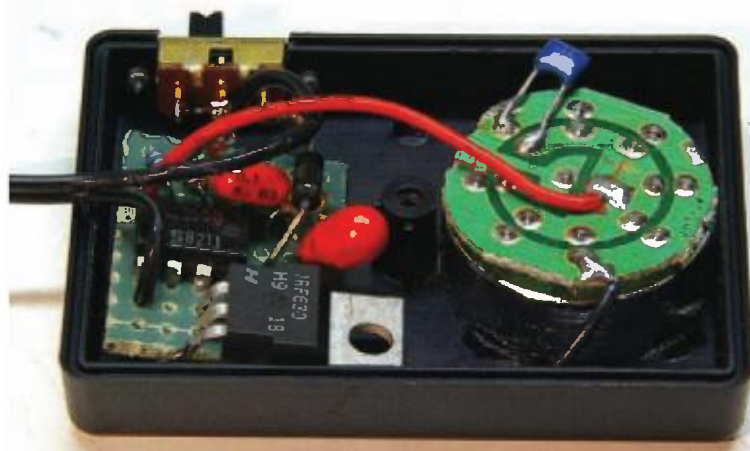
■ PHOTO 5. Through-hole circuitry inside the task light.
