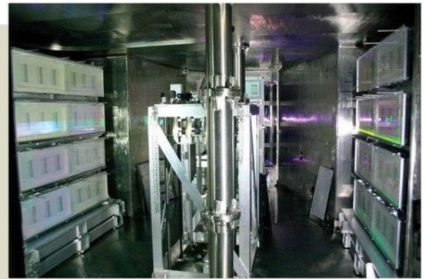
■ The ILE pulse compressor delivers 2,000 trillion watts.
