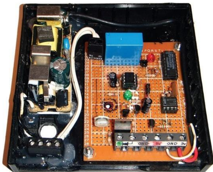
■ FIGURE 4. Everything mounted in the modified modem housing.
