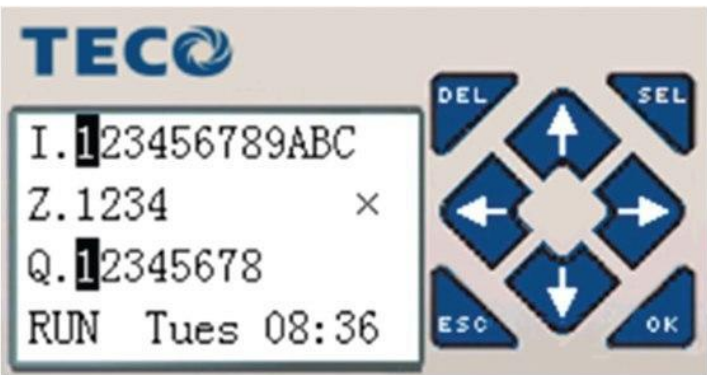
FIGURE 4. Status display shows I01 and Q01 energized.
