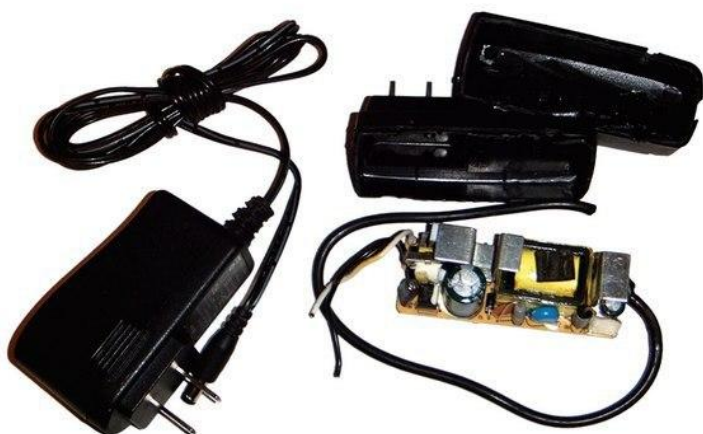
■ FIGURE 5.A wall wart supply — before and after.
