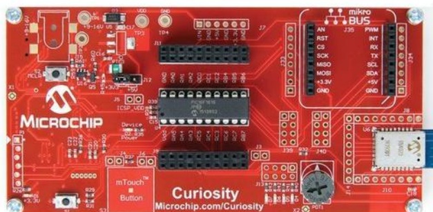
■ Photo 4. I've opted to solder in a raw RN4020 Bluetooth Smart radio module instead of plugging in an RN4020 click . The RN4020 is a breeze to mount and solder manually.
