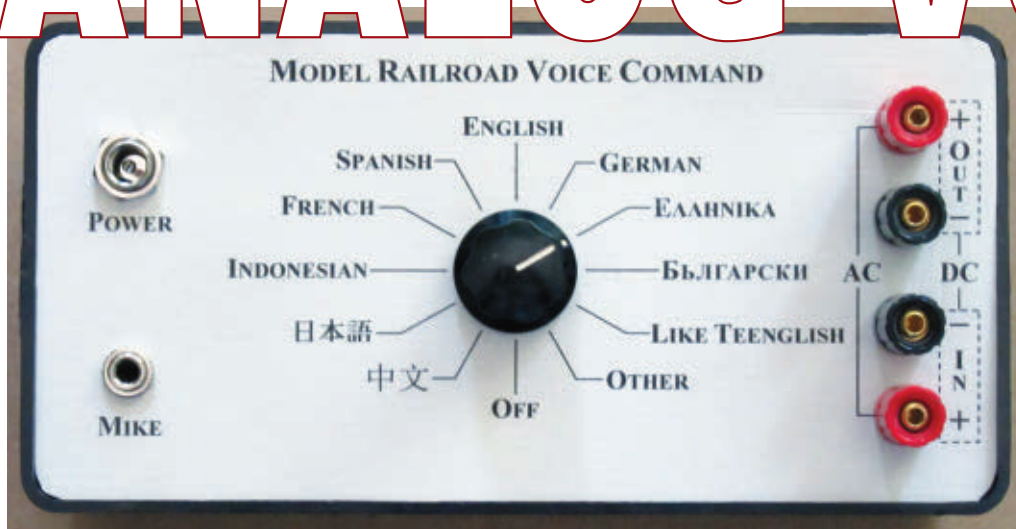
■ FIGURE 1. The completed Train Voice Command unit. The rotary switch serves as an off-on switch; otherwise, it is not connected to anything and has absolutely no electronic function. Its purpose is amusement, and to mystify onlookers and make them believe that the train control can understand various and diverse languages.
