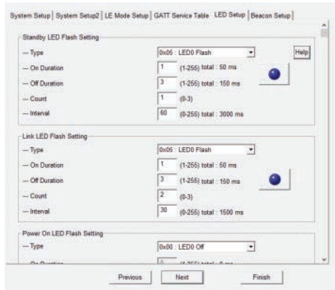
■ SCREENSHOT 9. These timing values determine how the blue status LED blinks when advertising and when connected.
