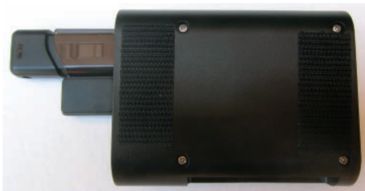
FIGURE 4. Bottom of the media center case. Note the Velcro strips which hold it to the back of the display in both our RV and home TV. Securing it to the back of the display means it takes up zero additional space.
