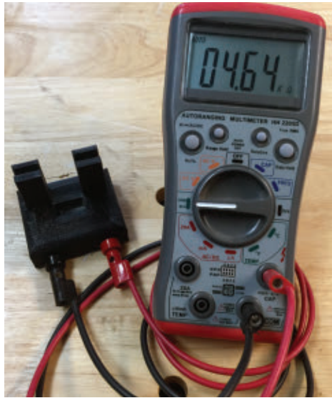
■ FIGURE 7. Testing a resistor.
