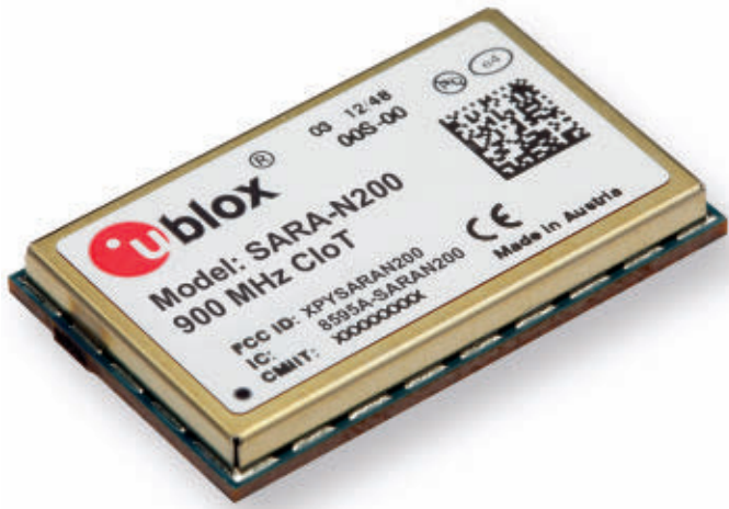
■ FIGURE 2B. The U-blox SARA-N2 module is an NB-IoT transceiver in a 16 x 26 mm package.
