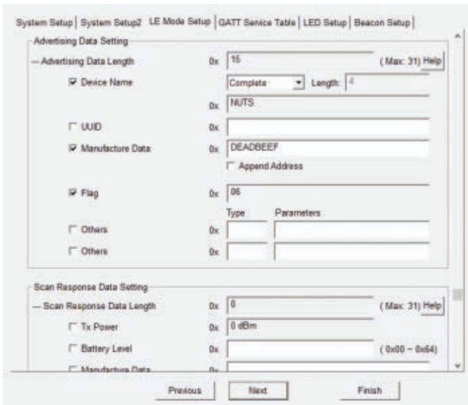
■ SCREENSHOT 7. Our BLE central (iPad) will scan the Ether looking for BLE peripheral advertisements. Once a BLE advertisement is received, it is up to the BLE central to initiate the connection.
