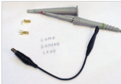
Figure 1 A standard oscilloscope probe has a ground lead that can pick up noise.
