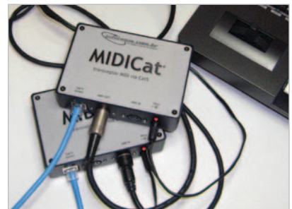
Figure 1 You can test the completed MIDI drivers with a 100m Category 5 cross cable.
