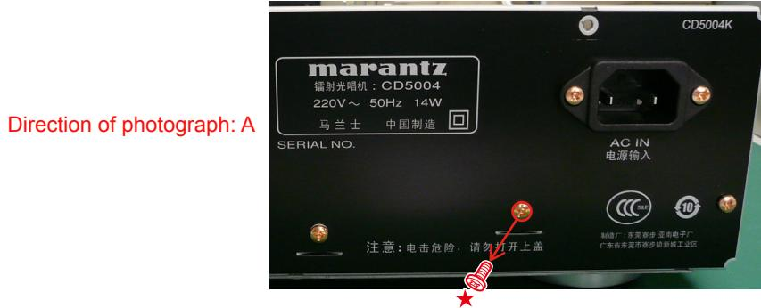
(2) Remove the screws. Disconnect the connector wires. Cut the wire clamp band.
