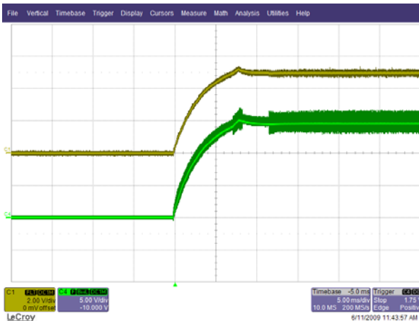
Figure 18 – Start-up Profile, 265 VAC. Upper: V_{5V} , 2 V / div. Lower: V_{14.5V} , 5 V, 5 ms / div.
