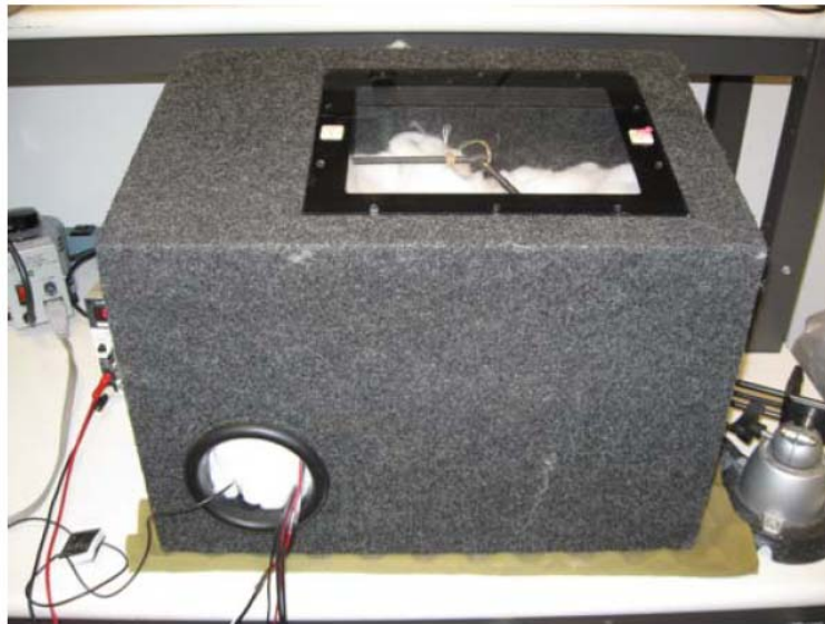
Figure 32 – In-House Audio Test Chamber (L: 20" x W: 13" x H: 13").
