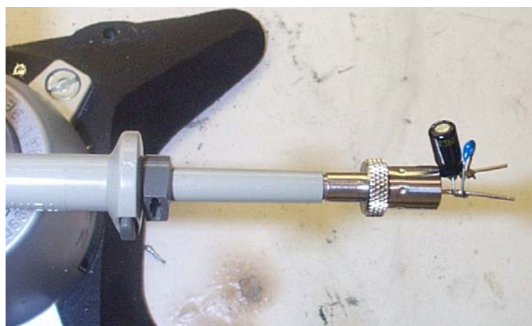
Figure 27 – Oscilloscope Probe with Probe Master ( www.probemaster.com ) 4987A BNC Adapter (modified with wires for ripple measurement and two parallel decoupling capacitors added).
