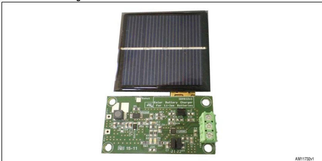
Figure 1. STEVAL-ISV012V1 demonstration board
